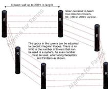
The towers are completely wireless. They have a built-in battery pack, which is kept charged by a small solar panel on the top of the tower. The battery will keep the unit going for up to a month without sunlight, and for satisfactory operation, the towers need only a couple of hours' sunlight a fortnight.
